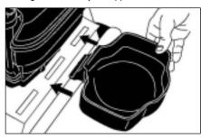
Step 1 Slide the detergent tray into one of the slots of your choice. Secure the tray to the frame by fastening the screw.
