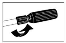
Step 2 The wand must be set in the low pressure (-) position to apply detergents.
