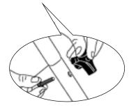
Step 3 Insert the handle into the frame. Align holes, insert bolt, and tighten with knob.
