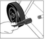
Step 6 Disconnect the high pressure hose from the high pressure outlet and engage the gun safety lock.
