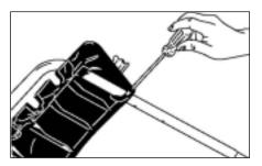
Step 2 Align the holes of the accessory rack to the handle and fasten the four screws.
