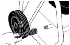
Step 4 Connect high pressure hose to high pressure outlet.
