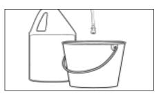
Step 3 Fill a container with Kärcher detergent. Place the filter end of detergent suction tube into the container. Be sure to adjust the filter by turning it to the desired detergent intake.
