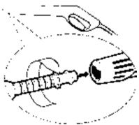
**Step 2** Insert the spray wand of your choice into the trigger gun. Press in against the spring tension and twist into the locked position.
