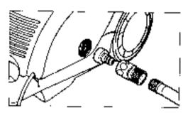
**Step 3** Connect garden hose to unit's water inlet using the quick connect adapter.
