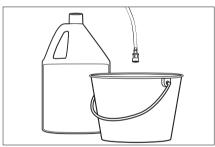
detergent. Place the filter end of detergent suction tube into the container.
